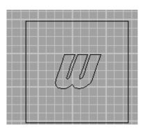
**3.** If needed, fillet the sharp corners of the letter to fit your mill bit's <u>radius</u>. Next, check all tight spaces with a circle the size of your chosen bit to make sure that the bit will fit into those spaces. ((Make sure that the **Join** option is yes at the fillet prompt. Try to go in a clockwise or counter clockwise pattern when filleting.))
