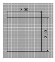
2. Create a letter and place it in the center of the rectangle and save as "Original letter" ((Before saving, size the letter so that the mill bit will fit into the small places. The bit is usually a .0625 diameter single fluted router bit.))
