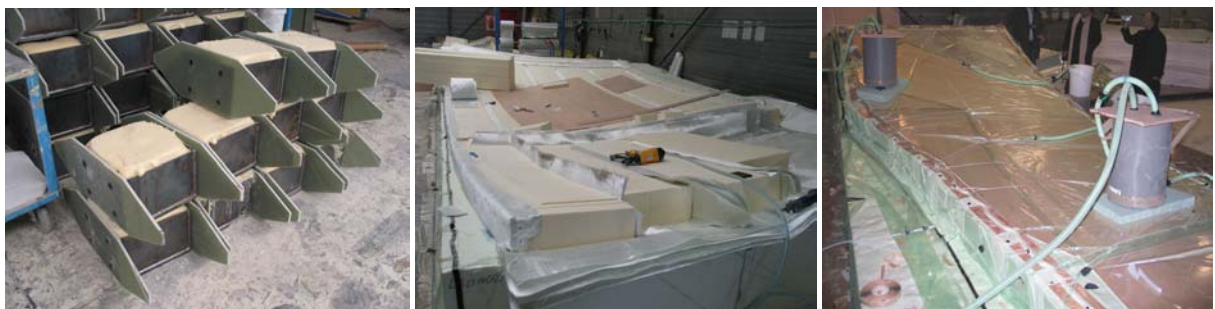
Figure 34. Inserts to be placed in the sandwich in order to make a connection between the roofs and the columns. The foam inside the inserts prevents polyester to gather and thus creating concentrated extra weight.
